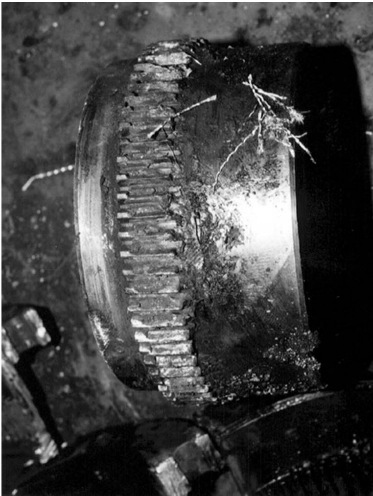
FIGURE 1.8 Worn gear coupling hub.
